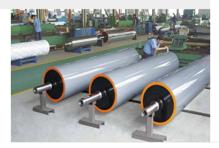
High speed of casting film production line means very high rotation speed of the roller, and this requires precise dynamic balancing, high and balanced heat exchange efficiency;
